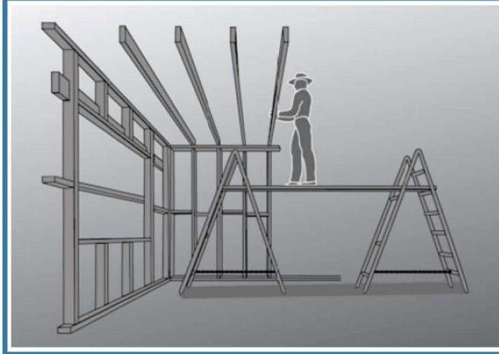
FIGURE 12 Installing ceiling or upper level floor joists
