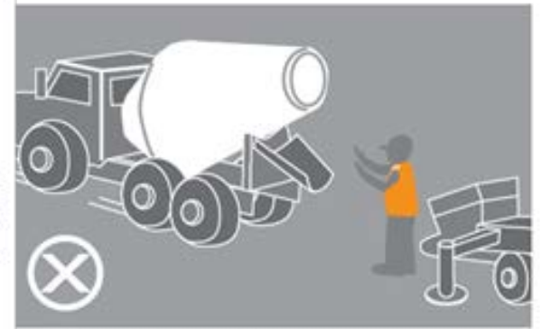
Keep clear when truck is reversing into position, don't stand between truck and hopper
