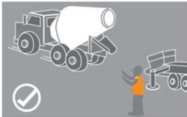
Keep clear when truck is reversing into position, ensure you remain in driver's view.
